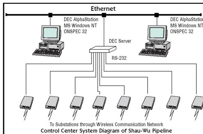
Two ONSPEC systems (Windows NT) are used in the central control room in Wulumuqi. Real-time data from the field is transferred to the control room via wireless communication devices. The ONSPEC system monitors and controls the status and operation of all the equipment of the pipeline with geographical maps, system diagrams, graphics, trends, data, and reports.
